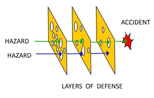
The model shows "holes" in each barrier to reflect the fact that no control is perfect. This is especially true when considering human factors.
