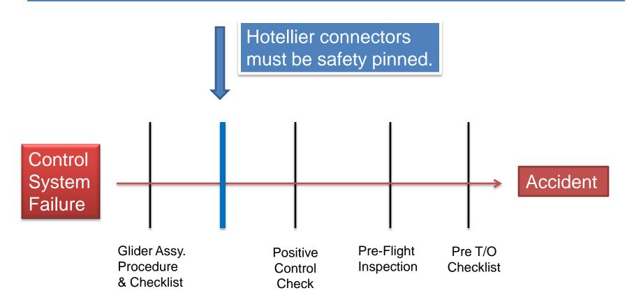
The added layer of defense guarantees discovery. If not properly installed, the glider will fail the Positive Control Check.
